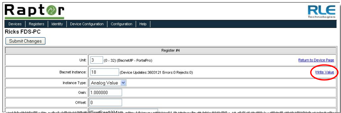
Figure 3.14 BACnet “Write Value” Link
