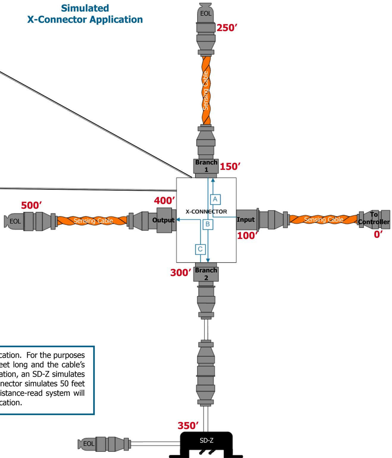
This drawing represents a simulated X-Connector application. For the purposes of our example, each piece of sensing cable is 100 feet long and the cable's resistance is 2.8 ohms/foot. In a distance-read application, an SD-Z simulates 50 feet (15.24m) of cable and each branch of a X-Connector simulates 50 feet (15.24m) of cable. The diagram shows you how a distance-read system will calculate the distance at various points along the application.
