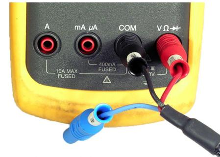
**Important!** - Do not connect the leads to the wrong inputs, or you will blow the multimeter's internal fuse.
