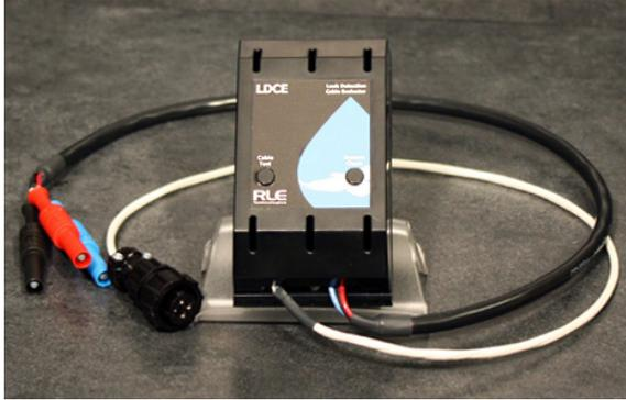
Thank you for purchasing a SeaHawk LDCE leak detection cable evaluator. This guide outlines device operation. Before you use the LDCE, check the RLE website to ensure you are using the most recent version of our documentation.
