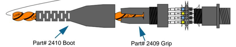
7 Screw the grips onto the plug and receptacle, and tighten by hand. Screw the boots onto the grips, and tighten by hand.
