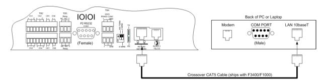
Figure 2.5 F110 Ethernet Connection to a PC on a Subnet
