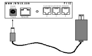
Figure 2.3 5VDC Power Supply Connection
