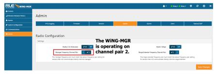
If you should need to change the WiNG-MGR back to channel pair 1, return to this web page, click the toggle button to select channel pair 1, and click the Save Changes button. Then verify the WiNG-MGR is communicating on channel pair 1 by checking the System LED and ensuring it blinks blue (900MHz) or purple (868MHz).
