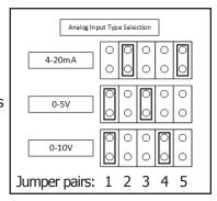
If your input is 0-5V, place the jumpers on pairs 1 and 3. If your input is 0-10V, place the jumpers on pairs 1 and 4.
