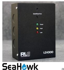
Thank you for purchasing a SeaHawk LD1000 single-zone leak detection controller. This guide outlines device installation and operation. Before you install a LD1000 reference our website www.rletech.com - to ensure you are using the most recent version of our documentation.
