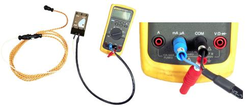
Connect the LDCE, the sensing cable, and the multimeter as shown.
