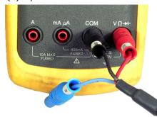
To test the LDCE's battery, connect it to the multimeter as shown.
