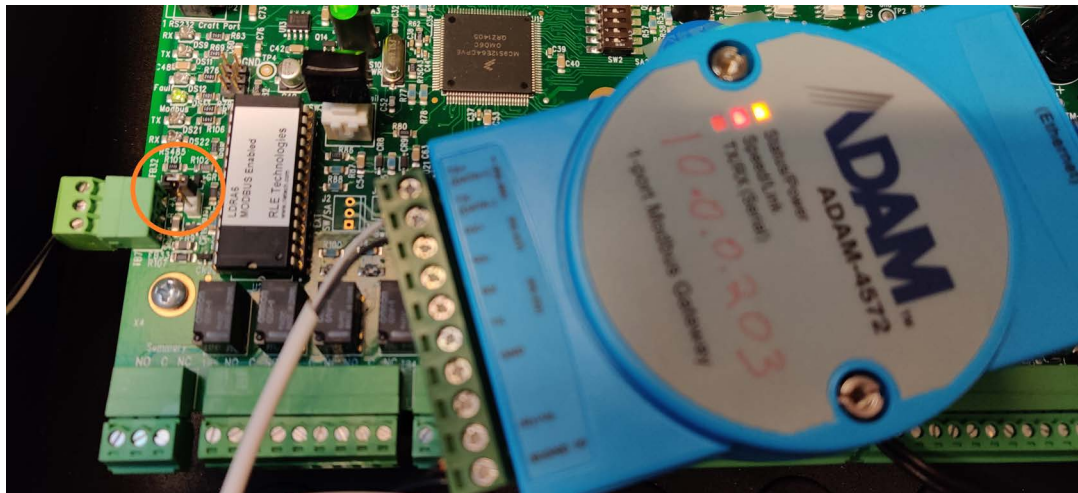
Image: Termination Resistance Jumper – Termination Disabled (Default)
