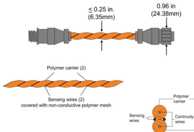
RLE Conductive Fluid Sensing Cable
