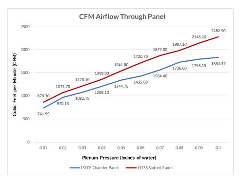
At RLE, we focus on CFM. We know the air that flows *through* the panel is more important than the open spaces cut into the top of the panel.
